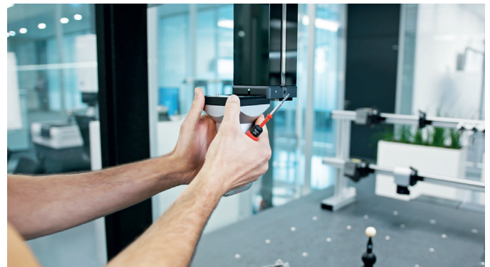
Step 2: Simple sensor removal thanks to dovetail mechanism
