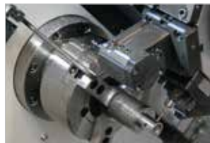
Chuck Air Blow (Upper Chuck)
