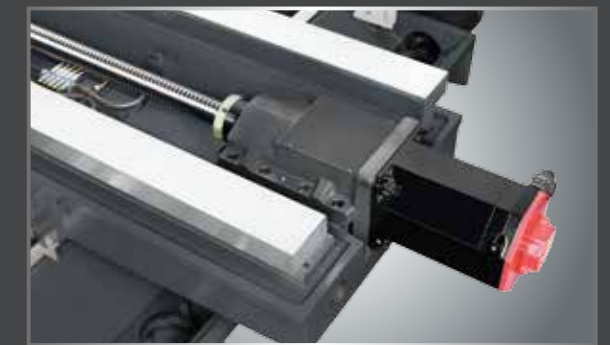
Direct-drive servo motor
