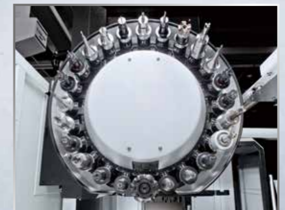
24T Disc type tool magazine
