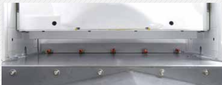
Bed Flushing Coolant
