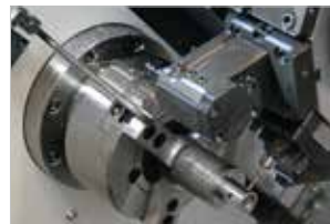
Chuck Air Blow (Upper Chuck)
