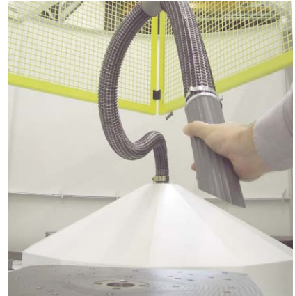
Workpieces can be cleaned with a wet vacuum cleaner. (Preparation)
