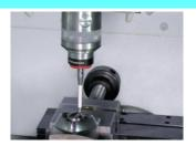
MARPOS T25S measuring probe with radio connection inserted in spindle HSK-A63, work piece scanning with automatic storage of data via measuring cycles. Receiver 8AO-CICMIRICWRI is included.
