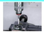
MARPOSS WRS T25S measuring probe with radio connection inserted in spindle BT40, work piece scanning with automatic storage of data via measuring cycles. Receiver 8AO-CICMIRICWRI is included.
