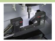
MARPOSS MIDA 75 Laser "light barrier", mounted on the machine table for probing of tool edges and automatic takeover of the values into the tool offset memory for further processing.
