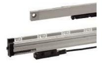
Linear measuring of position with "linear scales" to eliminate displacement (thermal growth) and increase machine precision. The pressurization of the scales prevents the penetration of dust or oil.
