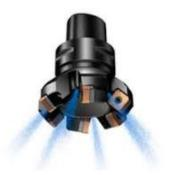
Optionally activation of coolant passage through spindle / tool via rotary coupling. High pressure pump 20 bar attached to 1 cartridge filter 60 micron or air blow 6 bar through spindle and tool
