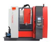
Control: **FANUC i0-MF**Advanced CNC control
