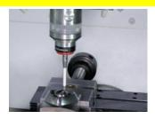
MARPOSS WRS T25S measuring probe inserted in spindle HSK-A63 with infrared connection 360°, work piece scanning with automatic storage of data via measuring cycles.
