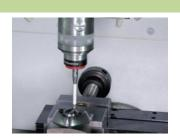
MARPOSS WRS T25S measuring probe with radio connection inserted in spindle HSK-A63, work piece scanning with automatic storage of data via measuring cycles.
