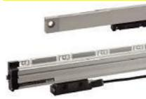
Linear measuring of position with "linear scales" to eliminate displacement (thermal growth) and increase machine precision. The pressurization of the scales prevents the penetration of dust or oil.
