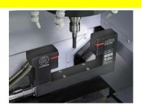
MARPOSS MIDA 75 Laser "light barrier", mounted on the machine table for probing of tool edges and automatic takeover of the values into the tool offset memory for further processing.
