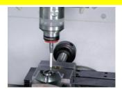
MARPOSS WRS T25S measuring probe inserted in spindle BT40 with infrared connection 360°, work piece scanning with automatic storage of data via measuring cycles.
