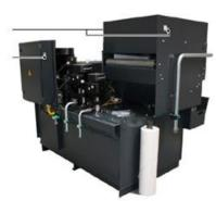
Drum paper band filter with 25 bar pump.
