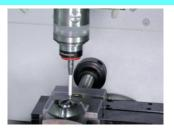
MARPOSS WRS T25S measuring probe with radio connection inserted in spindle ISO40, work piece scanning with automatic storage of data via measuring cycles. Receiver 8AO-CICMIRICWRI is included.
