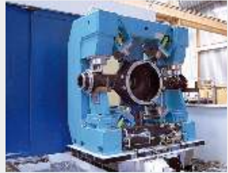
Jig with axle housing
