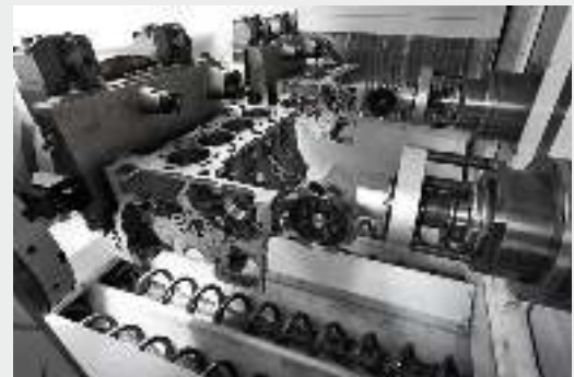
Machining a cylinder block with an angular milling head
