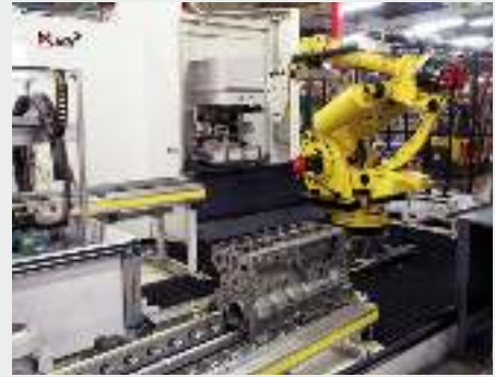
Transport of larger and heavier components with robots
