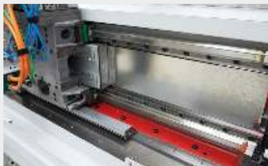
Z axis with linear drive
