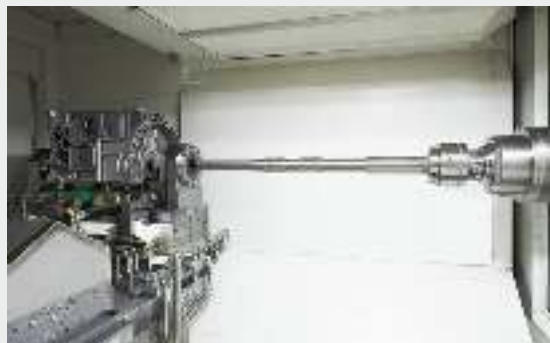
Crankbore machining on SPECHT® 600
