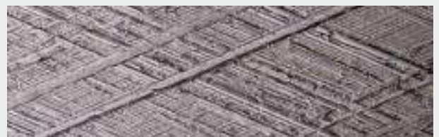
Magnification of a diamond-honed bore surface
