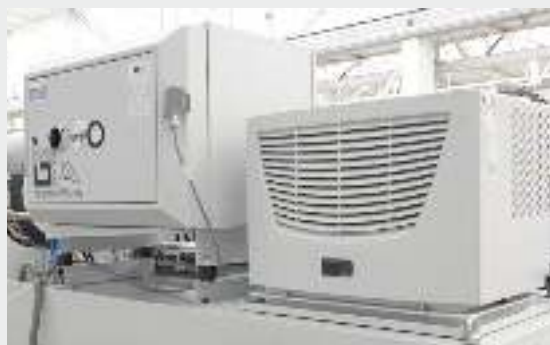
Oil and emulsion mist separators with cabinet cooling
