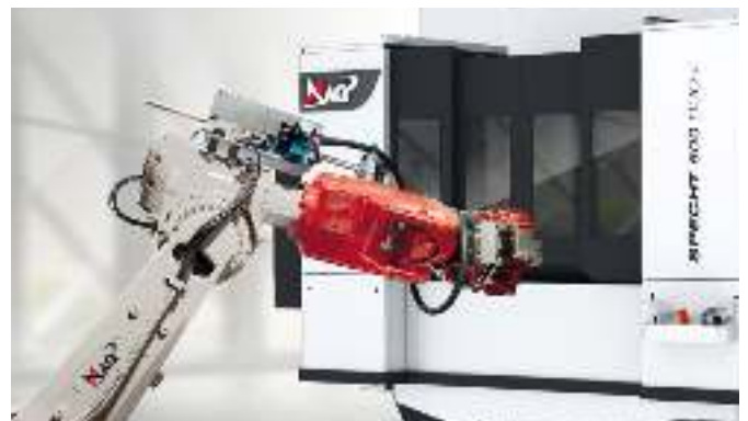
Robot loading on a SPECHT® 500 DUO+
