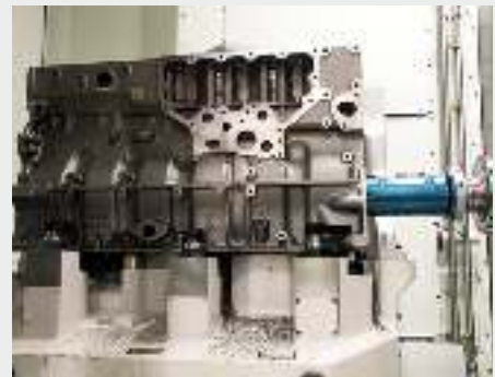
Machining crankshaft bore on a cylinder block
