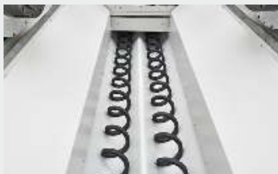
Chip tray with steep edges for good chip discharge also for MQL machining
