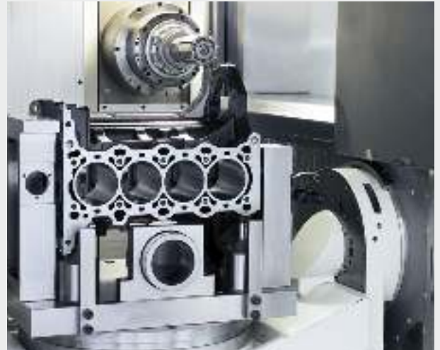
Honing a 4-cylinder crankcase
