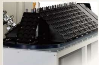
Work feeder (multiple pallets)
