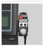
The MPG allows to manually wind forward or backward through a cutting path. This enables the operator to find the exact point along a cutting path from which to re-start cutting after a stoppage, or to simply locate a pre-cut part.
