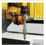
Should the cutting head inadvertently crash into a clamp/fixture, hit the edge of a work piece or an upturned part, the Break Away Head will detect the crash and automatically stop the machine.
