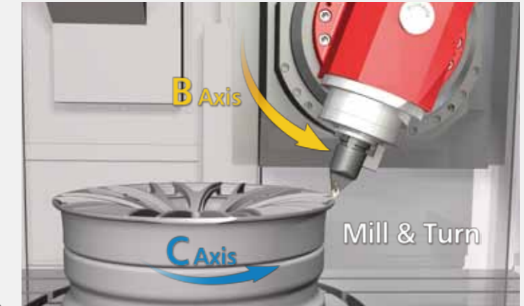
C axis rotary table can be separated from the machine. (BX300A / 500A / 700A / 900A)
