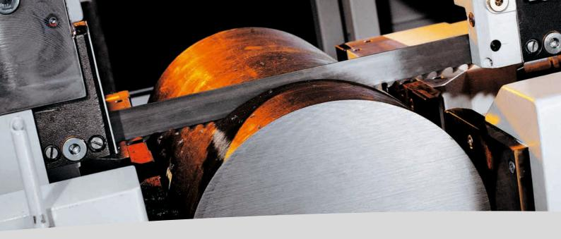
The new KASOTtec AC models combine solid heavy engineering with innovative control technology. A continuously adjustable electromechanical saw feed with two servomotors and ball screw spindles offer the best conditions for an efficient, precise sawing that is less wearing on the tools.
