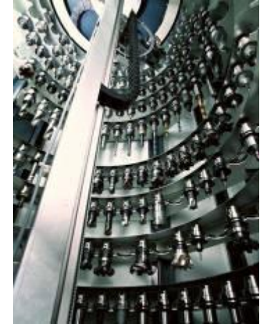
The tool tower is built as a circular rack The tool capacity is available in three stages 120, 170 or 220 places
