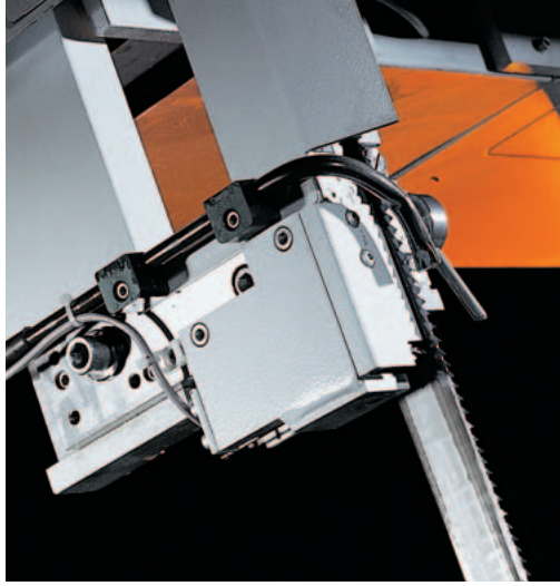
Hydraulic, electronically supervised saw blade tensioning. The height of the upper blade guide can be hydraulically adjusted.
