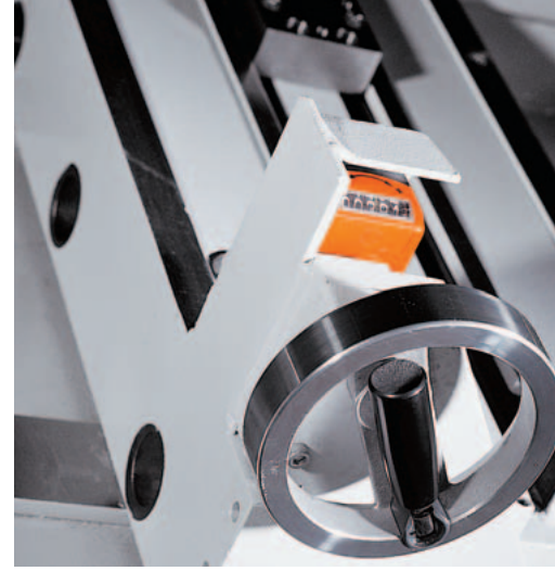
Mechanical measuring stop with digital display, fast and easy to adjust.
