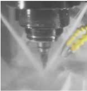
External coolant supply via two nozzles
