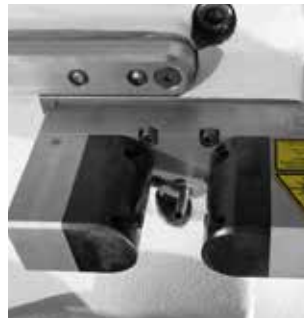
Air blow on C-axis positioned over laser system
