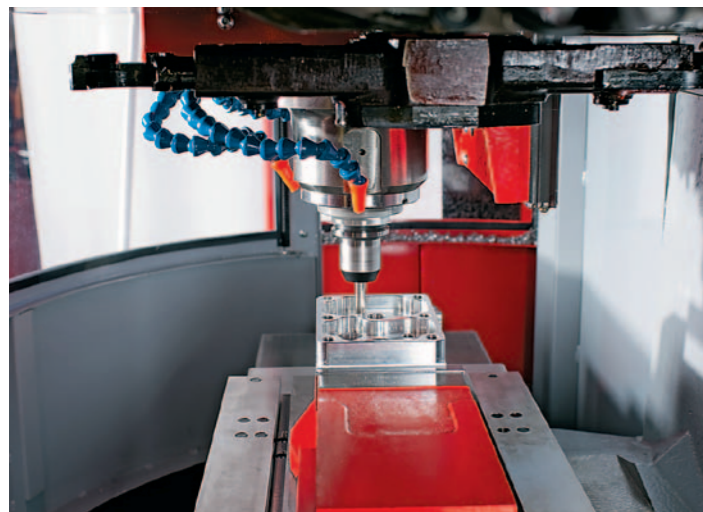
Dual-gripper arm and 'random' tool selection; mechanical spindle with high performance drive - 10000 rpm with 6,8 kW.
