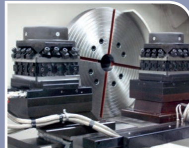
Combination of two 4-positions Sauter head-type turrets
