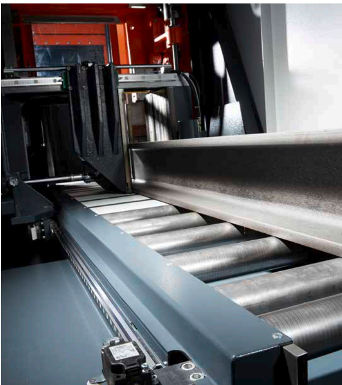
Material feed with 1.500 mm feed length (3.3, 4.6 and 5.6)
