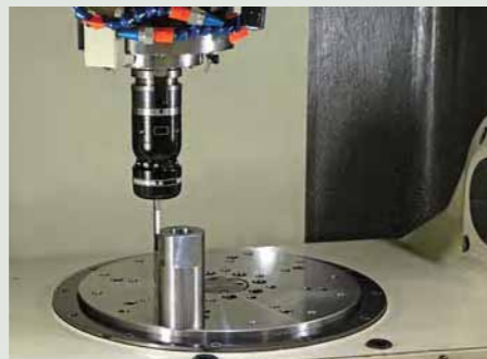
Measurement of C axis rotation center
