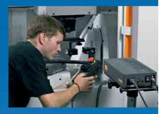
Every machining centre has been assembled in our air-conditioned assembly shops by qualified personnel, measured by means of a laser and submitted to extensive tests before delivery.
