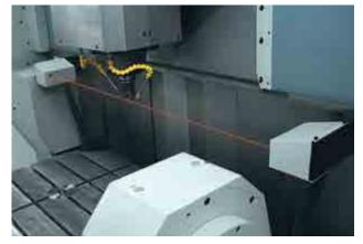
determining of the location, as well as workpiece plotting by means of the set-up probe.
