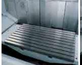
The lower table option brings 150mm more Z height for optimum machining conditions for large and bulky workpieces, or in connection with a dividing head.
