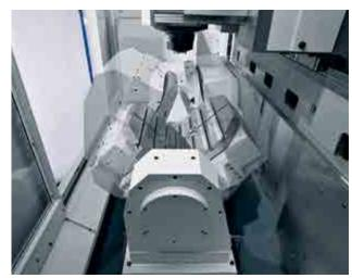
Swivel range from  $-100\ to\ +120\ enables\ optimum\ accessibility with the tool, especially for operations such as undercutting.$
