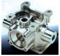
Example of a 5-side machining in regulated operation
