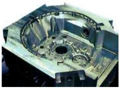
Example for 5-axis simultaneous machining
