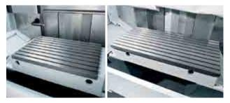
Standard table for workpieces up to 1.6 t. It is available in two different lengths: 900mm and 1300mm (for VCP 1000 Duro) x 600mm width. These flat tables have 9 T-slots for the secure clamping of workpieces suitable for the large working area.
