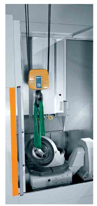
Access for crane loading and unloading is built in. The roof of the complete machine enclosure opens simultaneously with the sliding doors.
