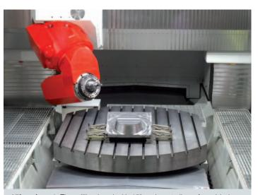
$15^{\circ}$  undercut. The milling head with  $15^{\circ}$  undercut allows for added value in complete machining in one setup.
