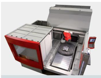
**Floor grid.** The floor grid inside the work space facilitates unloading and loading as well as the setup. Workpieces are easily accessible from each side.
