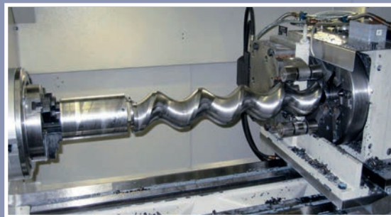
▲ Installation of whirling unit
