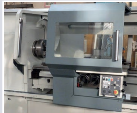
Additional control panel with hand-wheels installed on support
