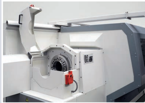
Second spindle nose with complete interlocked covers.
