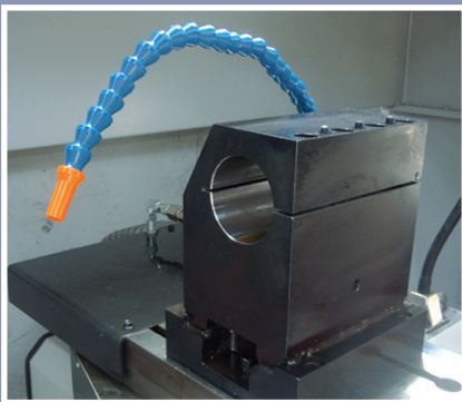
▲ Boring bar attachment mounted on cross-slide T slots
