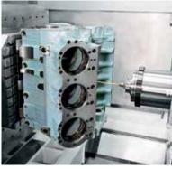
NC rotary and pivoting unit and tool tower magazine as option.
