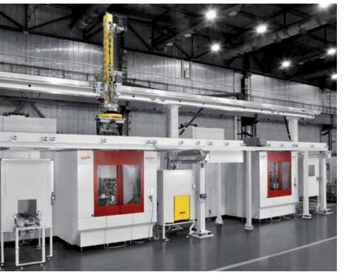
The machining centers HEC 500 / 630 / 800 Athletic have interfaces for the automatic workpiece, tool and information flow as a precondition for the integration into flexible production systems and production lines.
