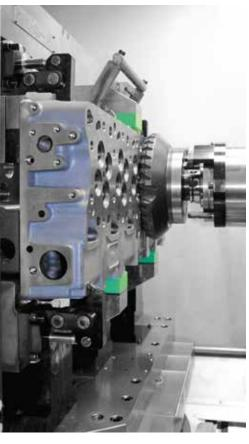
Machining of a crankshaft bore hole with 800 mm long boring bar.
