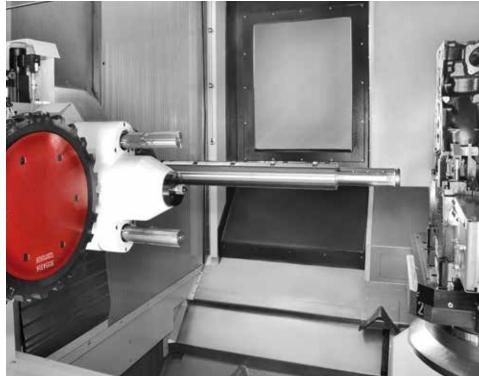
a higher tool demand, the machining centers can be equipped with the new modular tower magazines with a storage capacity of either 180, 270, 360 or 450 tools. Tools and additional quipment with a diameter up to 340 mm, a length up to 800 mm and max. 50 kg unit weight can be stored.
