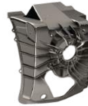
减震塔 Damping tower
