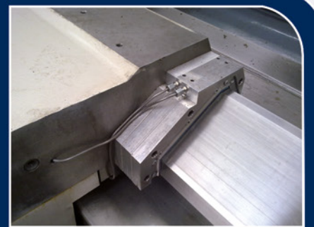
Double scrappers with compressed air for special guide ways security against grinding powder.
