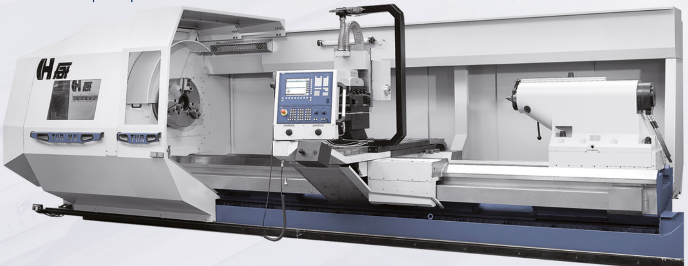
▶ Special headstock with high powerful motor and additional planetary gearbox. With this solution it is possible to obtain a torque of up to 32 000 Nm
