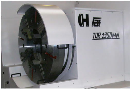
▶ Dual nose spindle with a 450mm diameter bore
