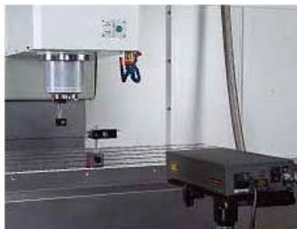
• Laser inspection is applied for every machine after installation to ensure perfect quality
