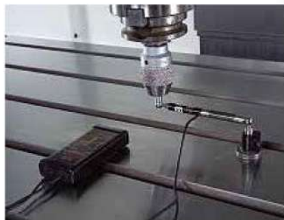
• High precision ball bar circle inspection
