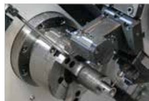
Chuck Air Blow (Upper Chuck)
