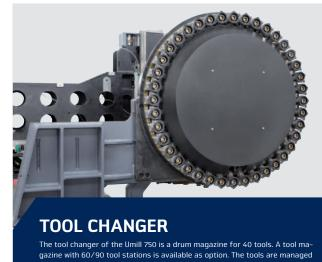
according to the variable tool station coding principle (random), which means that tools are always deposited in the first free magazine station for time reasons. Other tool changer sizes are available upon request.
