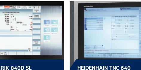
The Sinumerik 840D sl incl. Shopmill is an universal and flexible CNC system offering free contour programming, milling cycles for complex contours, fast reference point setting with touch probe systems, tilting of the working plane, cylindrical surface machining, 3D tool compensation
