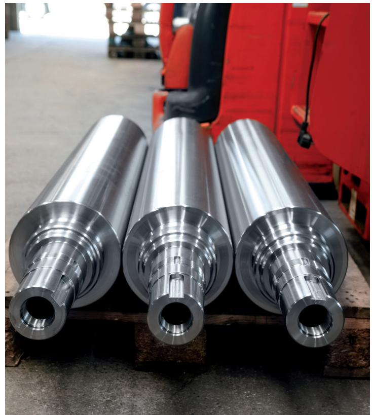
These drive shafts made of high-grade alloy steel with a diameter of 250 mm and a length of 2500 mm are completely processed using the Maxxturn 110.
