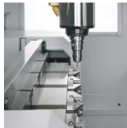
FZ 08 W Machining center with a workpiece changing device, for simultaneous loading and unloading of the machine.
