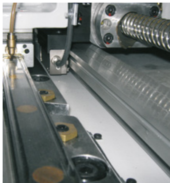
Highest precision: glass scales, digital drive technology and absolute path measurement systems allow high acceleration with equally high contour accuracy.
