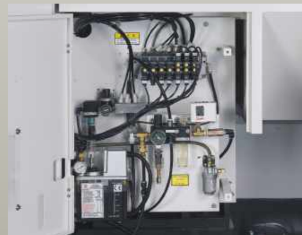
Hydraulic & Lubrication System(LU-620)
