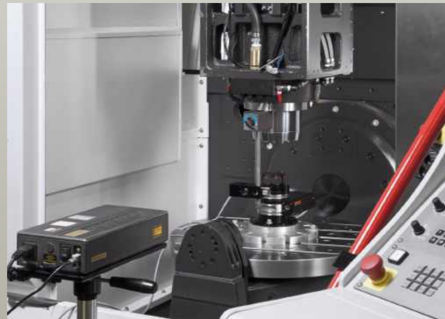
■ Worktable Center Calibration w/ Heidenhain TS740. High Precision Touch Probe & Standard Calibration Ball with Heidenhain Measurement Software can detect error value of the worktable and compensate to ensure Worktable Precision.
